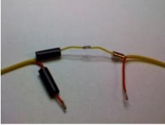
2. Place a splice barrel and short length of meltableinner shrink wrap on the wires. Lay the CHT and type-K extension loops over each other.
