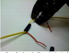
4. Crimp the splice barrel with a crimping tool (use a crimping tool with a grip for non-insulated terminals – the ones that have a cradle on one side and pierce a small hole on the other).
