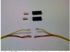
1. Strip the CHTs and make little loops with the ends. Do the same with the type-K extension wire. Prepare the splice barrels and heat shrink.
