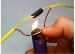
5. Slide the meltable-inner heat shrink over the splice and heat with a heat gun or lighter.
