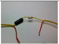
3. Slide the splice barrel over the parallel loops.
