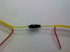
6. That is a solder-free, airtight and airless parallel thermocouple splice. Repeat as necessary.
